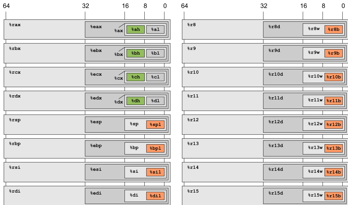
Figure 7. The arraignment of the different sized registers on the x86-64 architecture. Eight new 64-bit integer registers %r8...%r15 have been introduced and the old 32-bit registers have been extended to 64-bit versions. The byte registers highlighted with green background can only be accessed by using old instruction encoding of x86-32. The byte registers highlighted with red background are only available with REX encoded x86-64 instructions.
